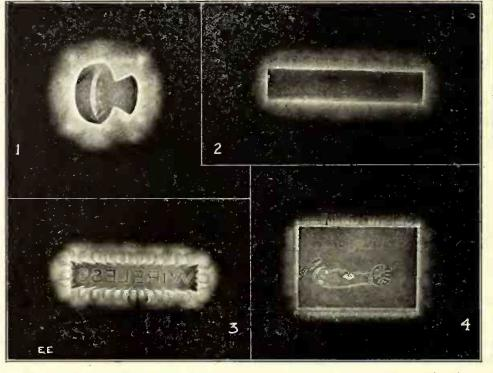
Some Out of the Ordinary Spark Pictures. (1) Made from Electrotype of Microphone, (2) Steel Rule, (3) Electrotype of "Wireless," (4) Zinc Line Cut of Arm and Hand.
