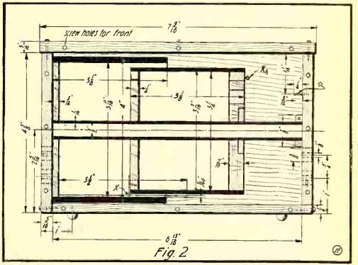
Fig. 2. Sidewise Sectional View of Coupler, Showing Primary and Secondary Coils. end of the wire from the outside into one hole and bring it out the other, leaving the loose end 6 inches long for connection. It is best to run the wire over a series of spools on spikes pounded into a flat board
