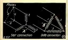
Alternating Current Circuit Hook-ups, at the Star Connection; at "B," Delta. at "A"
