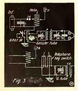
Fig. 3. Simplified Transmitting and Receiving Radio Hook-ups.
