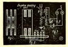
Making a Duplex Loading Coil.
