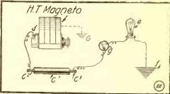
Electric Light From High Tension Magnetos.
