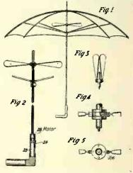
stem, as is evident. This shaft con-nects with a miniature electric motor 28, which receives current from a small flashlight type battery 29, in the handle of the umbrella. A push button 34 controls the battery cur-rent to the motor. The expense in making up this arrangement and also considering the gross efficiency, and especially the small "breeze producing power" in this case, does not seem to warrant at all the ex-pense in making up such an ar-rangement. angement.
