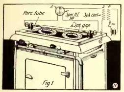
Fig. I. "Jump" Spark Applied to Gas Range.
