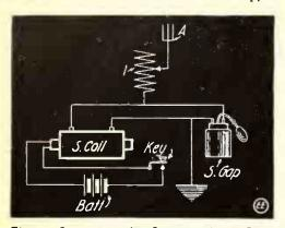
Fig. 1. Connections for Compressed Air Spark Gap.
