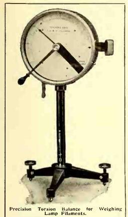
weighing extremely light bodies, but its principal application is in connection with the incandescent lamp industry. In the manufacture of incandescent lamps it is essential that the filament possess certain characteristics, one of which is that its length and, therefore, its weight shall be uniform within certain predetermined lim-While high accuracy is, of course, its. requisite, the instrument must at the same time be rugged; and these two features are embodied in this instrument.
