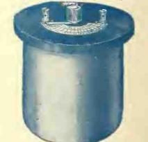
Note these specifications: The case is one piece of polished aluminum 4" in diameter and 4" high. It may he filled with oil with-out leakage, and this increases its capacity approximately five times. There are 31 aluminum plates, 16 station-ary and 15 rotating. These are fastened to a polished fibre top which rist tightly over the case. The top is provided with a celluloid scale, poluter, knurled knob and binding posts.
