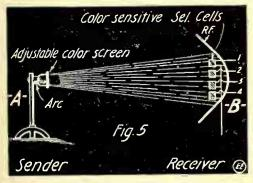
Fig. 5. Using the Selenium Cell for Wireless Control.
