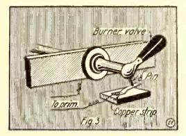
Fig. 3. Detail of Automatic Gas Stove Igniter Attachment.
