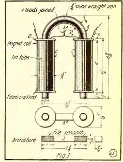
Fig. 1. Parts of Powerful Battery Magnet.
