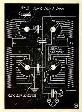
Modified Hook-up and Construction for Cohen's New Wireless Receiving Set. Dr.
