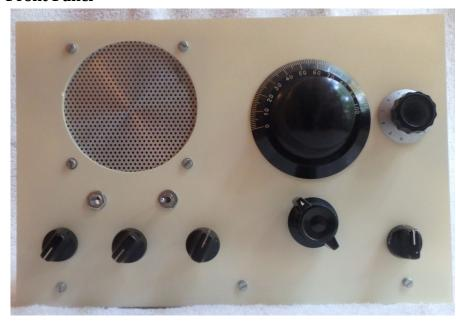
Bottom row, left-to-right: Audio gain & on/off switch RF attenuator pot Antenna coupling Band-switch Regeneration control
