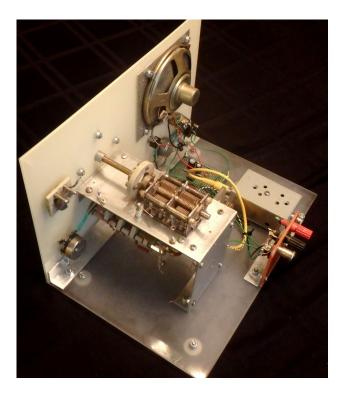
The band-switch is mounted beneath the L-shaped bracket. Above it, and hidden in this view, is the RF portion of the receiver.
