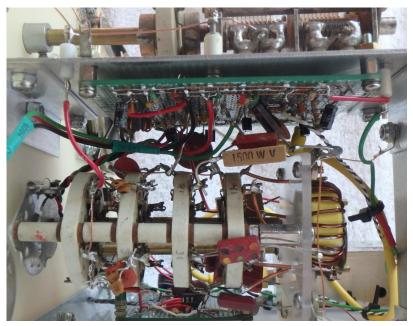
The antenna is coupled to the inductor via a link on the inductor. Too many turns on the link winding may adversely affect the regeneration. I kept removing turns until there was only one. In the end, I added a variable capacitor in the antenna link as well. There were no more turns to remove! I used a similar variable cap in the antenna link of a regenerative receiver I built many years ago.
