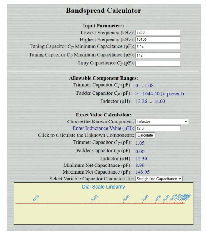
Situation 2: Same parameters, but here using an SLF cap: Really spreads it out. It works well. Note: Tuning range is wide. Almost 4:1 Close to the 3:1 range of the AM broadcast band.
